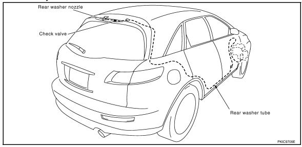
Removal and Installation of Washer Nozzle
