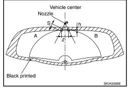
• Insert a needle or suitable tool into the nozzle hole and move it to adjust the spray position.
