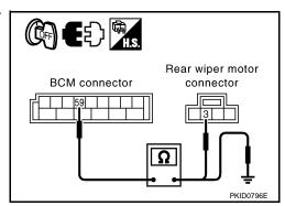
Check continuity between rear wiper motor harness connector and ground.
